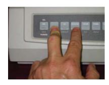
If the name of the dealership is printing too low (below the black line), make sure the "Sel" light is off, then press and hold the two buttons as shown to adjust...
